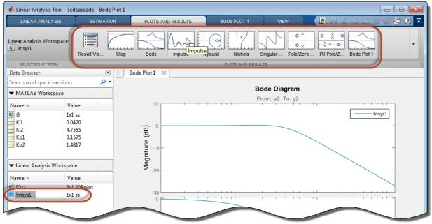
To access the Linear Analysis Tool from a Simulink model, in the Simulink Editor, select **Analysis > Control Design > Linear Analysis**. See the following topics for more information about using Linear Analysis Tool for:
