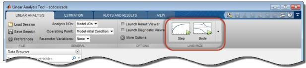
• The new **Plots and Results** tab also provides a gallery of plot types for creating additional plots of system responses. In the **Plots and Results** tab, select a dynamic system model from the MATLAB Workspace or the Linear Analysis Workspace. The plot gallery updates to reflect the available plots for the type of system you have selected. If the system you select was created in the Linear Analysis Tool session, the result viewer is also available in the plot gallery.
