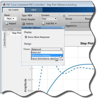
You can still use the **Response Time** and **Transient Behavior** sliders to further adjust the balance between reference tracking and input disturbance rejection.
